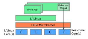
Fig. 1. A thread detached from L<sup>4</sup>Linux running on a separate core.
