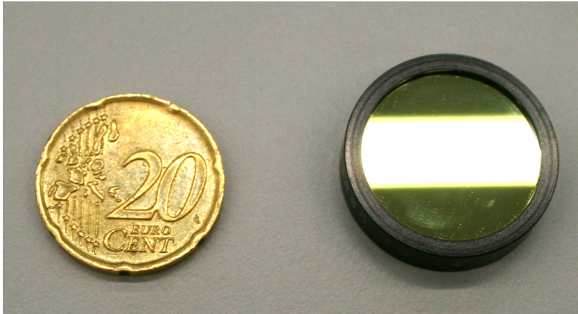
Figure 4.12.: Thorlabs bandpass that has been tested with cameras in the Virtable.
