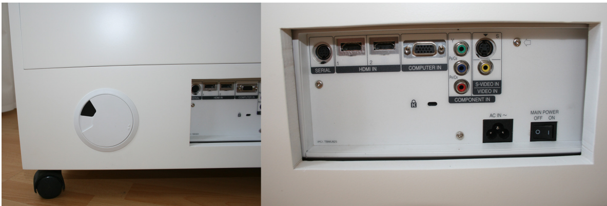
Figure 4.14.: Openings in the Virrtable's body: cable channel (left), projector connections (right)
