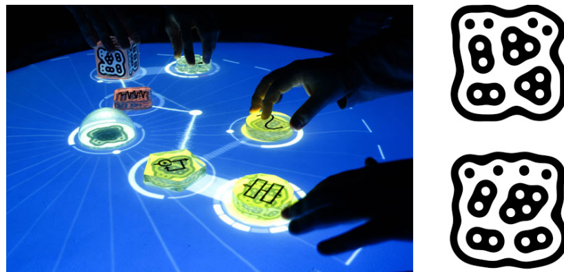
Figure 3.13.: On the left: the reactable in use. Source: [rea08a]. On the right: reactTIVision fiducials. Source: [rea08c]
