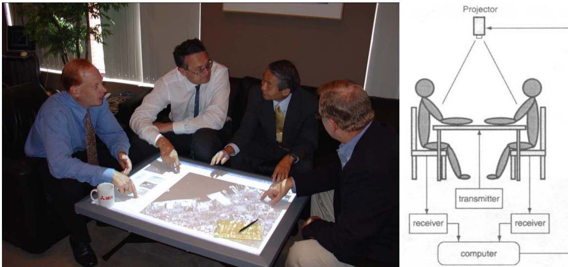
Figure 3.15.: DiamondTouch table in use and schematically. Source: [DL01]
