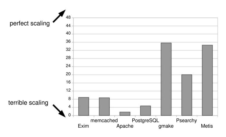
Y-axis: (throughput with 48 cores) / (throughput with one core)
