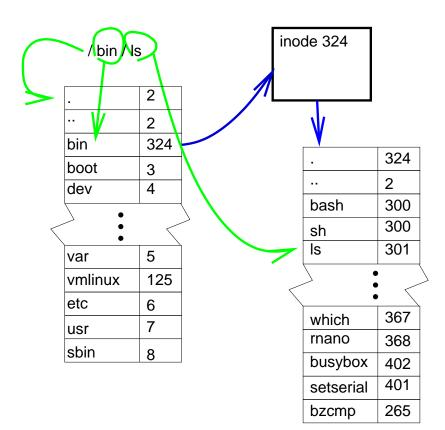
Linux has many different filesystem types. Each has its own directory layout. Pathname lookup is abstracted in the Virtual FileSystem (VFS) layer. Traditionally, looking up the name to inode (namei) mapping has been slow (done naively, it involves reading a block from the disk for each pathname component); Linux currently uses a cache to speed up lookup. This cache in turn has become a scalability bottleneck for large SMP systems.
