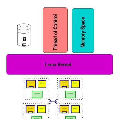
The POSIX process model works by inheritance. At boot time, an initial process (process 1) is hand-crafted and set running. It then sets up the rest of the system in userspace.
