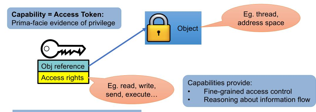
Any system call is invoking a capability: err = cap.method( args );
