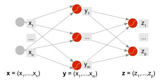
In the following, we focus on the most basic type of neural network, the **multi-layer perceptron** (MLP).
