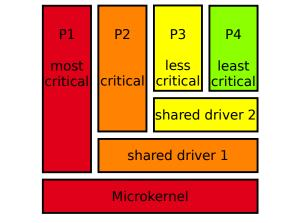
Shared drivers need to have *same* or *higher* criticality levels than their clients. Here, driver 1 is shared by {P2 .. P4} and has to fulfill P2's level.
